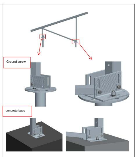
c.It's installed in the above mentioned installation explanation . And unification of the height and agreement of the installed height of the rail are secured by a size adjustment by a request on a drawing.
