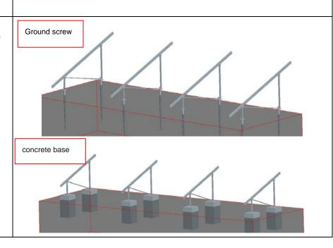
d.According to the drawings,connect the aluminum angle and support,Fixed tightly with M10\*80 hex bolt.
